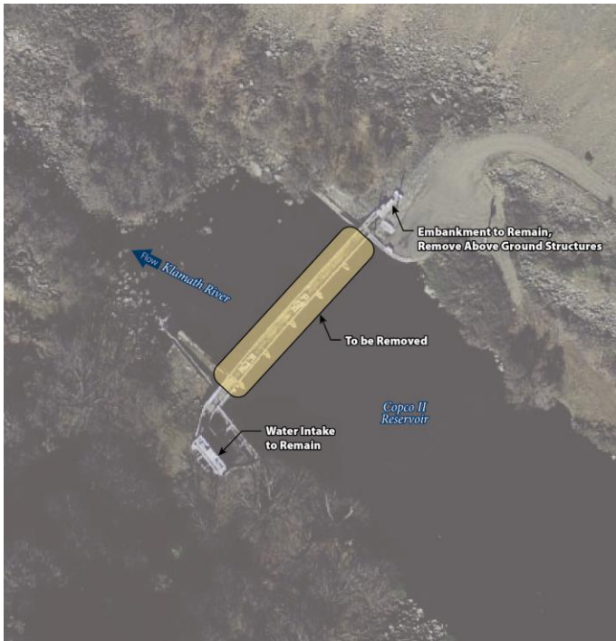
Figure ES-16: Partial removal of Copco 2 Dam would include removal of spillway gates, providing a free flowing river and allowing full volitional fish passage. Certain structures, including the water intake and embankments, would be retained.
