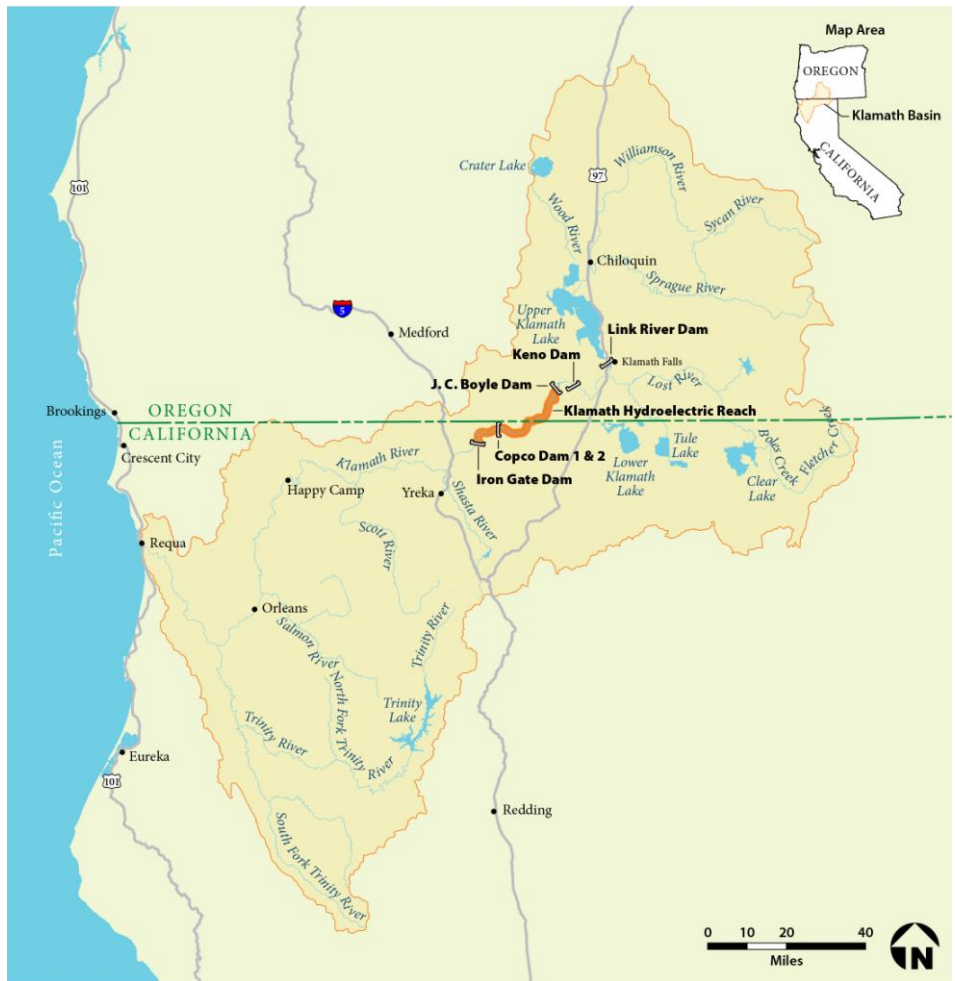
Figure 1-1: Klamath River basin map. J.C. Boyle, Copco 1, Copco 2, and Iron Gate dams would be removed under the KHSAs.
