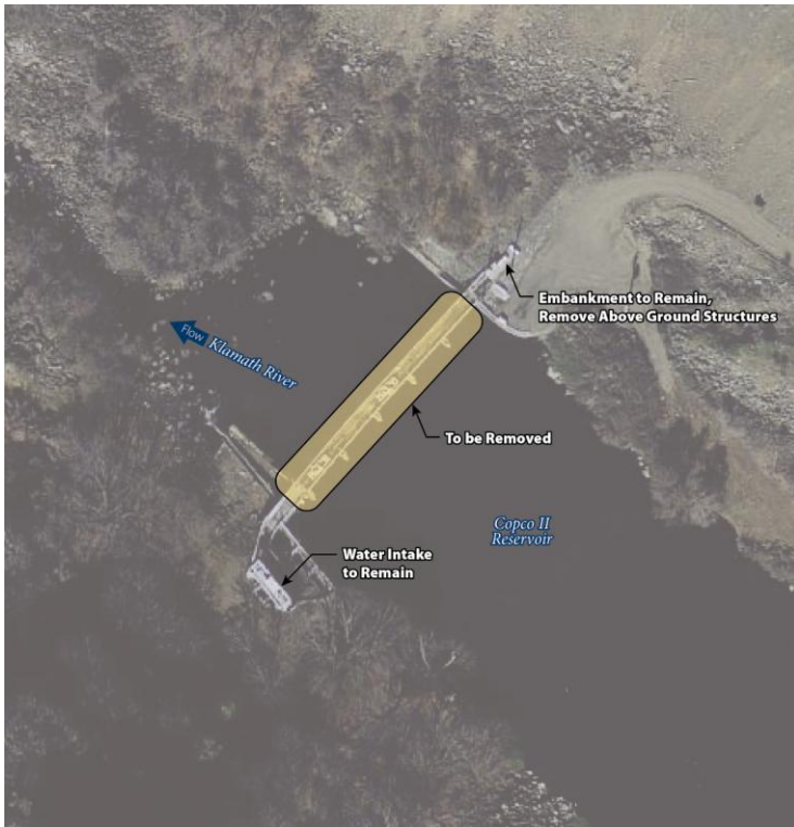
Figure 4.2-9: Partial Removal Would Provide a Free Flowing River and Allow Full Volitional Fish Passage. However, certain structures would be retained.
