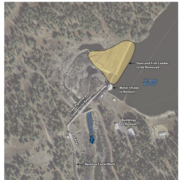
Figure ES-14: Partial removal of J.C. Boyle Dam would include removal of embankment dam and fish ladder, providing a free flowing river and allowing full volitional fish passage. However, certain structures, including the steel pipeline and supports, would be retained.
