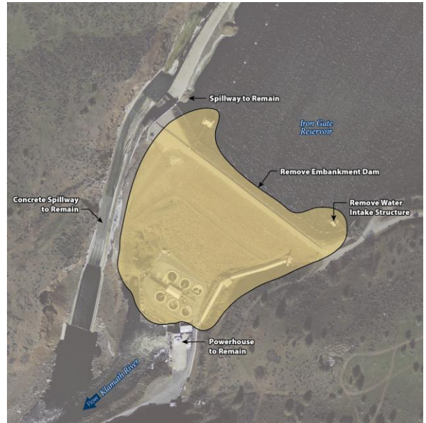
Figure ES-17: Partial removal of Iron Gate Dam would include removal of embankment dam, providing a free flowing river and allowing full volitional fish passage. Certain structures, including the spillway and powerhouse, would be retained.
