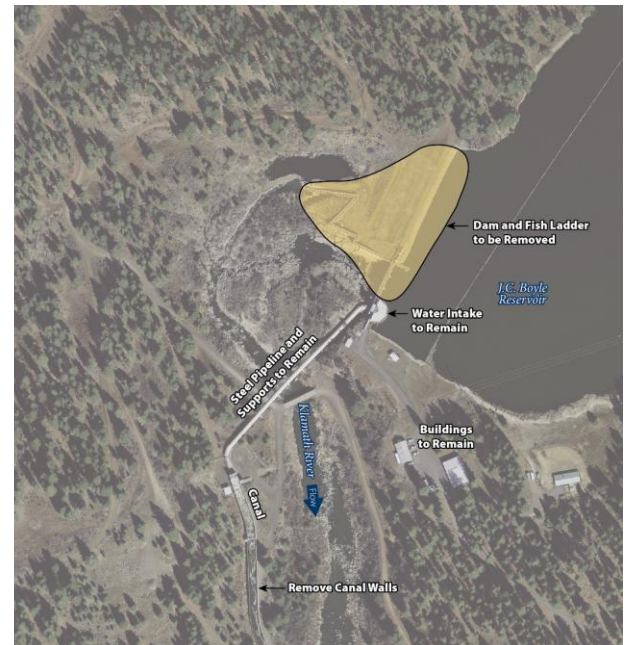
Figure 4.2-3: Partial removal would provide a free flowing river and allow full volitional fish passage. However, certain structures would be retained.
