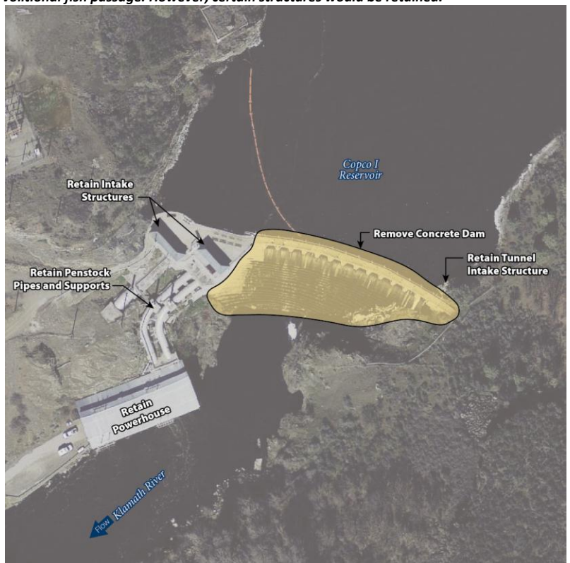
Figure 4.2-6: Partial removal would provide a free flowing river and allow full volitional fish passage. However, certain structures would be retained.
