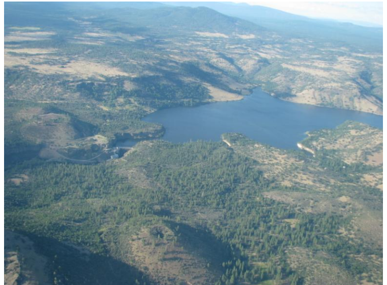
Figure 4.1-20: The relatively deep Copco 1 Reservoir experiences thermal stratification and results in low dissolved oxygen (from less than 1 mg/L to 5 mg/L) in reservoir bottom waters during summer and fall months. This poor water quality affects the Klamath River downstream of Copco 1 Dam.
