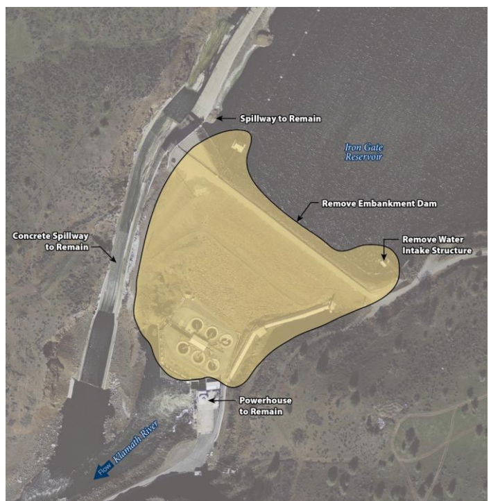
Figure 4.2-11: Partial removal would provide a free flowing river and allow full volitional fish passage. However, certain structures would be retained or retained and buried.
