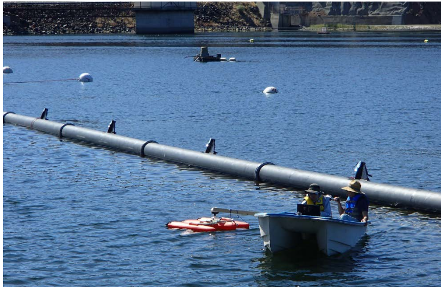
Figure 47. Acoustic Doppler Current Profiler Transect Measurement Along the Curtain in Iron Gate Reservoir in August 2015.
